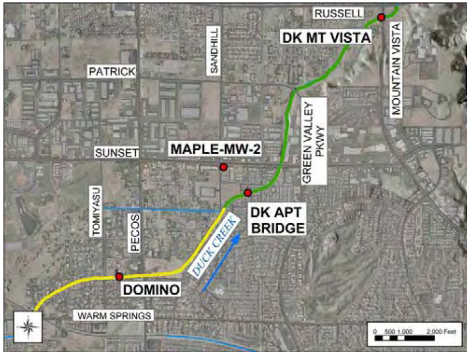
Figure 3. Map detailing sampling sites along Duck Creek. The Domino site is the start of perennial flow in Duck Creek. Lined channel highlighted in yellow, natural channel highlighted in green.
