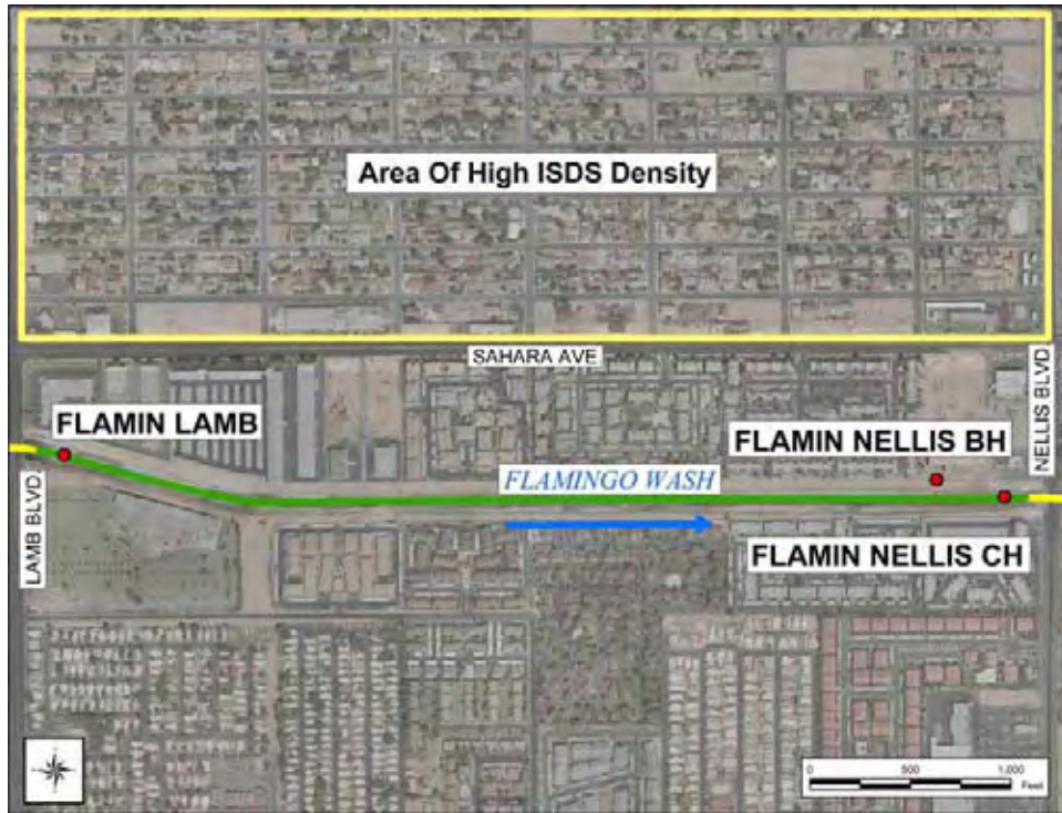
Figure 8. Map detailing locations of surface water sampling sites and borehole along reach of Flamingo Wash. Area of high ISDS density is in the north portion of the map. Many of the parcels located north of Sahara have registered ISDS. Lined channel highlighted in yellow, natural channel highlighted in green.
