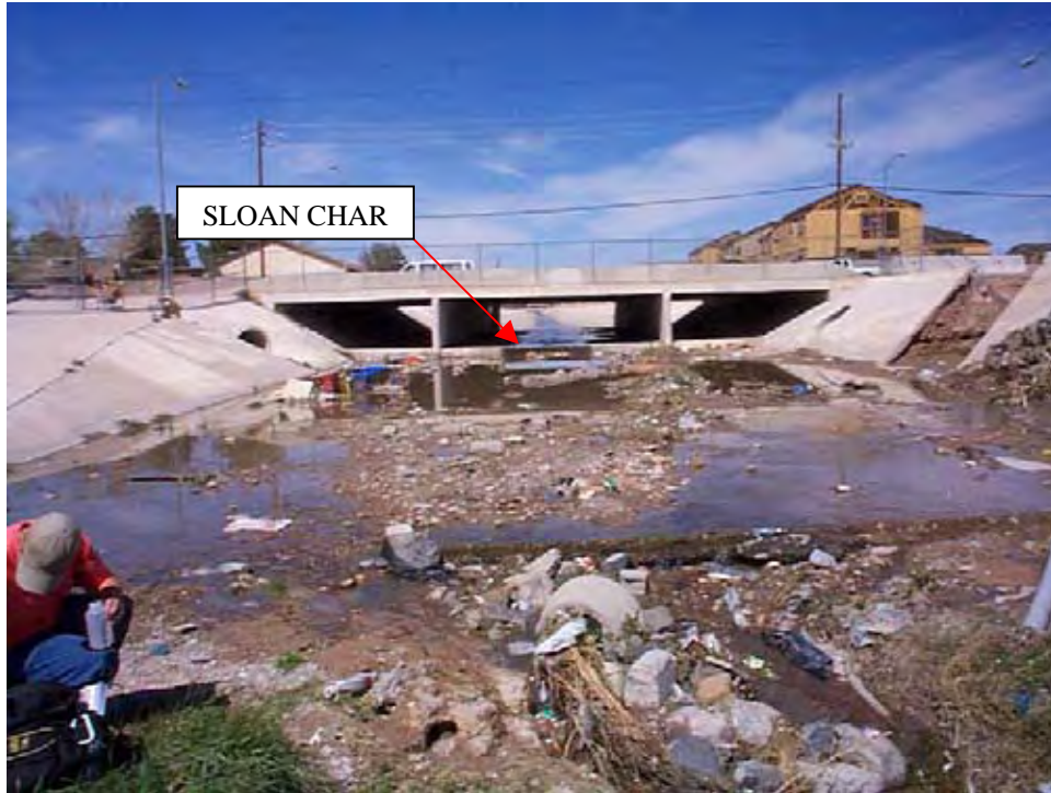
Figure 13. Photo detailing surface water sampling site on Sloan Channel at Charleston Blvd. Sampling is conducted under the bridge above the spill over (SLOAN CHAR).
